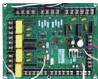
CZ-NS4P PCB for advanced functions in J and H Generation.
